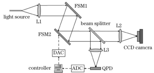
Fig. 2. Schematic of the experimental setup with L1, L2, and L3 lenses.
