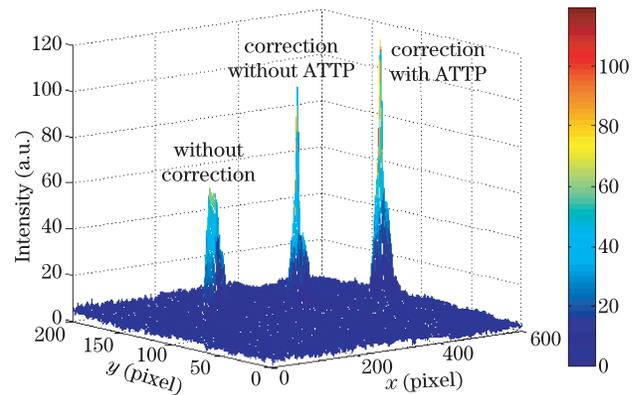
Fig. 6. Image energy distributions of three dimensions with and without corrections.
