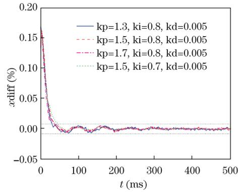
Fig. 5. Output signal of QPD using different control parameters with ATTP.
