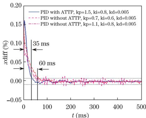
Fig. 4. Output signal of the QPD with and without ATTP.
