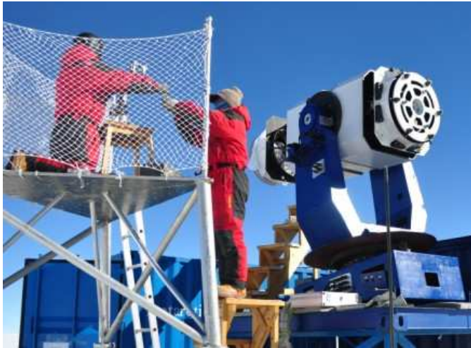
Figure 7. AST3-1 alignment at Kunlun station.
