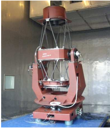
Figure 1. Winterization test of the whole telescope.
