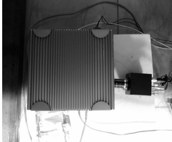
Fig. 4 Low temperature testing of Industrial control computer and CCD camera
