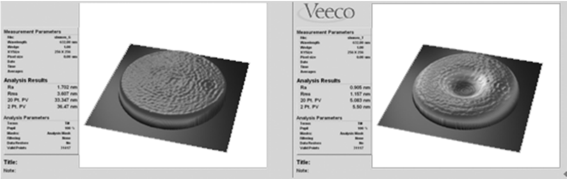
图 5 顺序分步消去法加工后的镜面面型与驻留时间 Fig. 5 Mirror surface ( left) after polishing with the method of sequential stepwise elimination and corresponding dwell time ( right)
