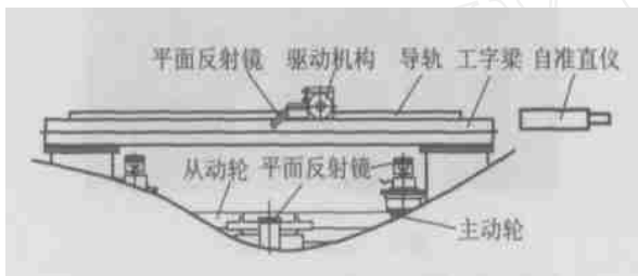
Fig. 3 Schematic diagram of skew angle
