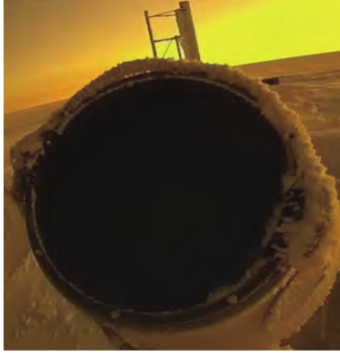
Fig. 1. The defrosting effect on the AST3-2 sealing window, showing a clear circular surface in the center and a visible accumulation of frost and snow along the edges.
