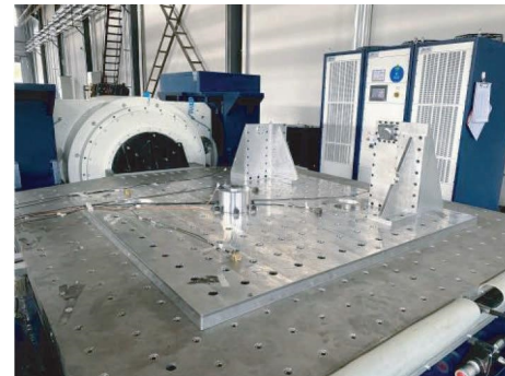
FIGURE 16: Test platform frequency sweep test.
