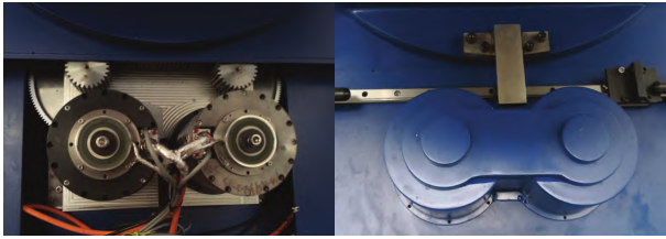
Fig. 4. Photographs of the fully enclosed gearbox used for AST3-3.
