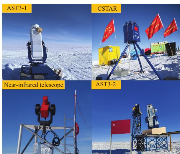
Fig. 2. Optical astronomical telescopes at Dome A in Antarctica. AST3-1, the first optical telescope in Antarctica with automatic pointing and tracking function. CSTAR, the first independently developed Chinese Antarctic optical telescope. The Near-infrared Telescope, filling the observational wavelength gap of 1.1–1.4 \mu\text{m} , installed in 2024. AST3-2, the largest aperture optical telescope operating at Dome A in Antarctica, installed in 2014.
