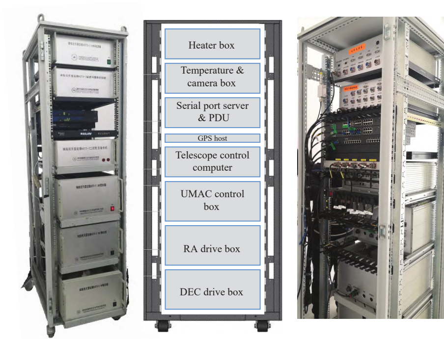
Fig. 9. The modularly designed telescope control cabinet, consisting of multiple modules with different functions, such as a controller module, driver module, and power supply module.
