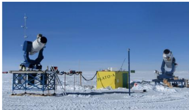
Fig2. AST3-1(right) and AST3-2(left) on Dome A
